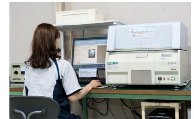
Measurement of components (energy dispersive fluorescent X-ray spectrometer)
