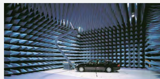
3D 測定系: 車輛用サイト Anechoic Chamber for Vehicle (3D Measurement Method)
