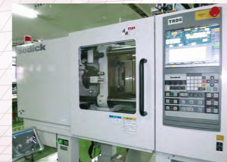
電動成形機による精密樹脂成形 Precision Resin Forming by Electric Micro Resin Molding Machine
