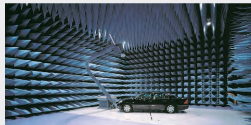
3D 測定系：車輦用サイト Anechoic Chamber for Vehicle (3D Measurement Method)
