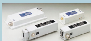
LNC (Low Noise Converter)
